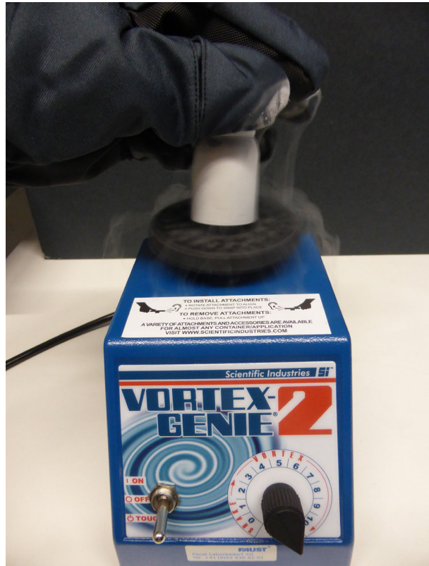
Fig. 5 Production of an inter-mixture of ice and dust by mechanical mixing on a vortex mixer. The ice and dust are kept at low temperature in an aluminium bottle that is regularly plunged into liquid nitrogen
