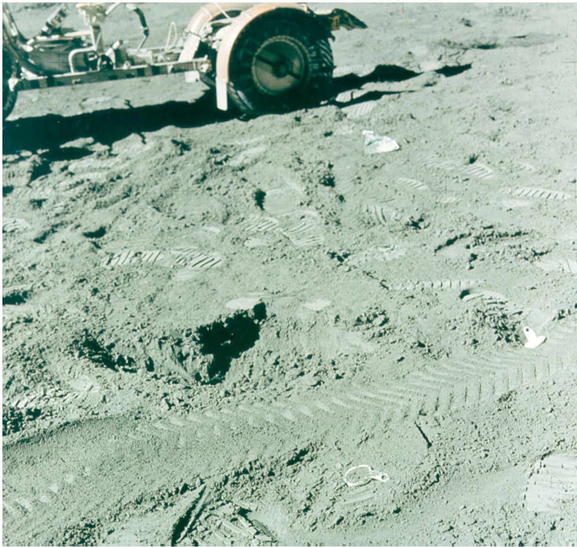
Figure 8: Another view of Soil Mechanics Trench - after the dirty deeds were done! NASA AS15-88-11874. Note the Teflon protective rings from the seals on the SESC (sample 15014).
