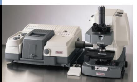
Nicolet FT-IR Spectrometer with Nicolet Continuµm XL Imaging System beamsplitter-locking mechanism allow easy access to the beamsplitter without breaking instrument purge and preventing beamsplitter fogging.
